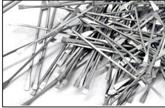
Figure 2.4: Steel Fibers - with flat heads
